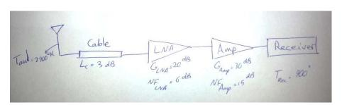
$$T_{eq} = T_{ant} + T_c + \frac{T_{LNA}}{\frac{1}{L_c}} + \frac{T_{amp}}{G_{LNA}} + \frac{T_{rec}}{G_{LNA}}$$
