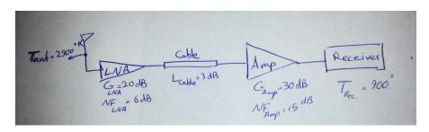
$$T_{eq} = T_{ant} + T_{LNA} + \frac{T_c}{G_{LNA}} + \frac{T_{amp}}{G_{LNA}} + \frac{T_{rec}}{G_{LNA}} + \frac{T_{rec}}{G_{LNA}}$$
