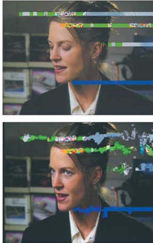
4. A single-bit error introduced in the middle of an MPEG slice (row of blocks) can cause a huge ripple through the end of the row (a). Subsequent video fields continue to use the corrupt video because of the interframe coding and motion vectors (b). The next Intra-Frame (approximately 500 ms) will clean up the video by starting a new anchor frame (JPEG picture).
