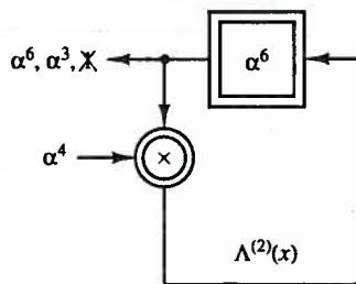
After the next clock the output will be  $\alpha^3 \cdot \alpha^4 = 1$  which is not equal to  $S_3 = \alpha^4$ .
