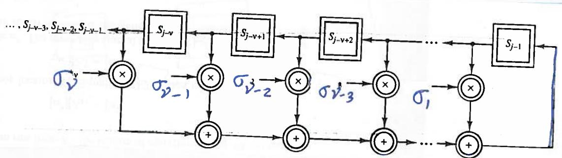
The problem of finding error-locator polynomial is then to find an LFSR of minimal length such that the first  $2t$  elements in the output sequence are  $S_1, S_2, \dots, S_{2t}$ . The coefficients of the filter are then the coefficients of  $\sigma(x)$ .
