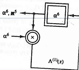
This works for the  $S_1 = \alpha^6$  as it outputs the content of the register, i.e.,  $\alpha^6$ .
