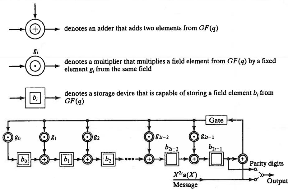
Encoding circuit for a  $q$ -ary RS code with generator polynomial  $g(X) = g_0 + g_1X + g_2X^2 + \dots + g_{2t-1}X^{2t-1} + X^{2t}$ .
