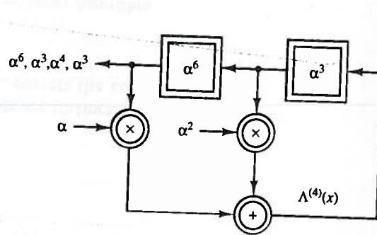
It is easy to see that this circuit outputs  $\alpha^6, \alpha^3, \alpha^4, \alpha^3$ , i.e.,  $S_1, S_2, S_3, S_4$ .
