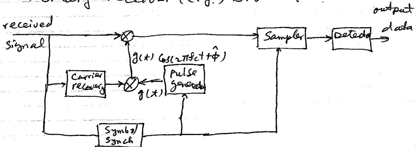
b) m-ary receiver (QAM or MPSK):
