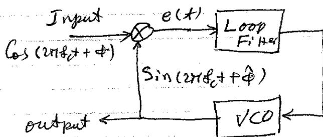
$$e(t) = \frac{1}{2} \sin(\phi - \hat{\phi}) + \frac{1}{2} \sin(2\pi f_c t + \phi + \hat{\phi})$$
