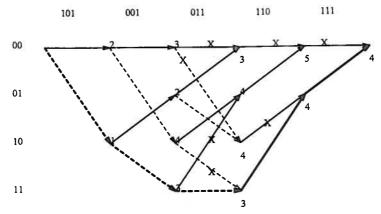
The decoded sequence is  $\{111, 100, 011, 100, 111\}$  (i.e the path with the minimum final metric heavy line) and corresponds to the information sequence  $\{1, 1, 1\}$  followed by two zeros.
