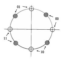
The signal points that may be transmitted at times t=2nT n=0,1,... are given with blank circles, while the ones that may be transmitted at times  $t=2nT+1,\ n=0,1,...$  are given with filled circles.
