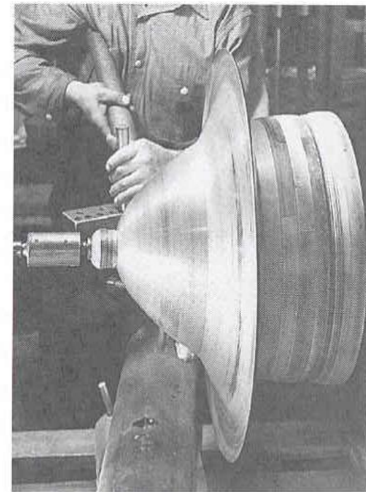
FIGURE 19-61 Two stages in the spinning of a metal reflector. (Courtesy of Spincraft, Inc.)
