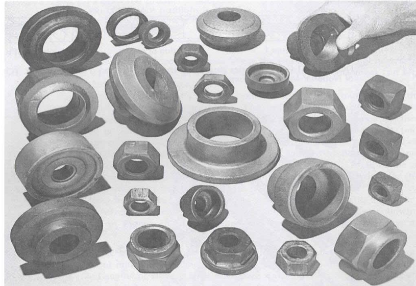
FIGURE 18-16 (Top) Typical four-step sequence to produce a spur-gear forging. The sheared billet is progressively shaped into an upset pancake, blocker forging, and finished gear blank. (Bottom) Samples of ferrous parts produced by automatic hot forging at rates between 90 and 180 parts per minute. (Courtesy of National Machinery Company.)
