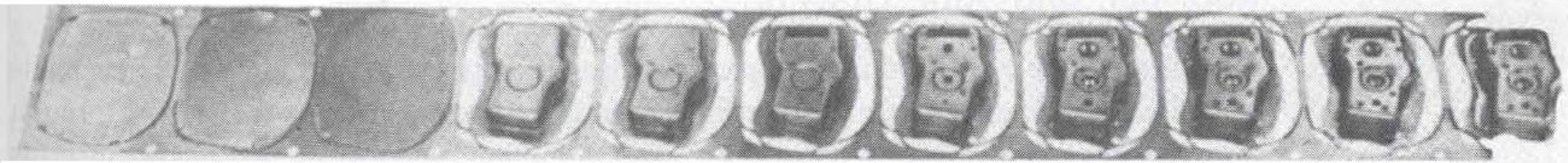
FIGURE 19-52 The various stages of an 11-station progressive die. (Courtesy of the Minster Machine Company.)
