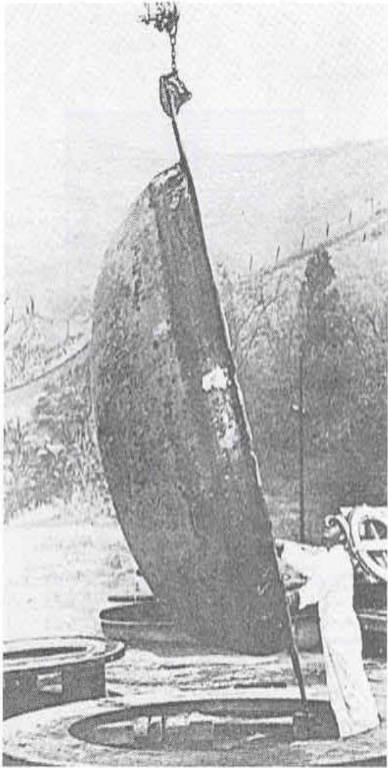
FIGURE 19-78 Explosively formed elliptical dome 10 ft. in diameter being removed from a forming die. (Courtesy of NASA.)
