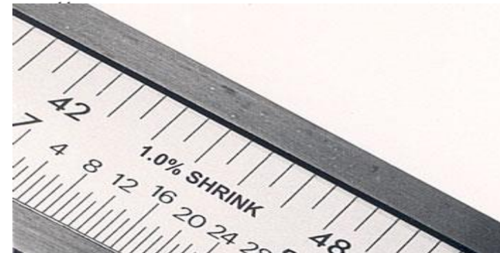
FIGURE 13-12 Various allowances incorporated into a casting pattern.
