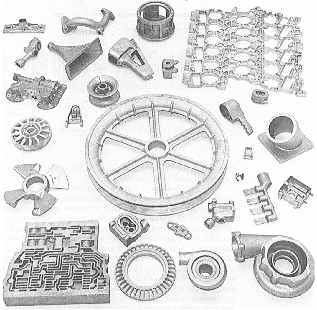
FIGURE 14-16 Some aluminum products produced by conventional sand casting. (Courtesy of Bodine Aluminum Inc.)
