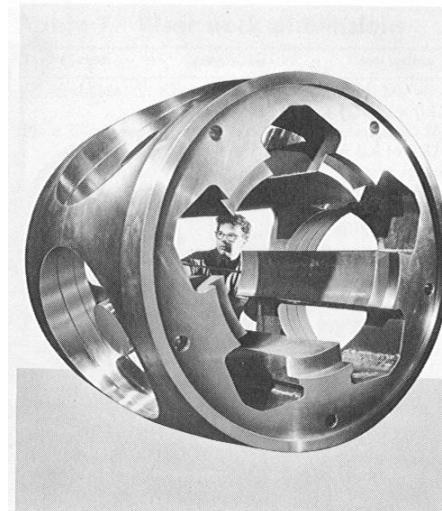
Fig. 27 Vertical centrifugally cast ship propeller hub for controllable-pitch propeller blades is made of nickel-aluminum bronze, weighs 8.44 Mg (18 600 lb), and measures 1575 mm (62 in.) in diameter and 1270 mm (50 in.) in length. Courtesy of Wisconsin Centrifugal, Inc.
