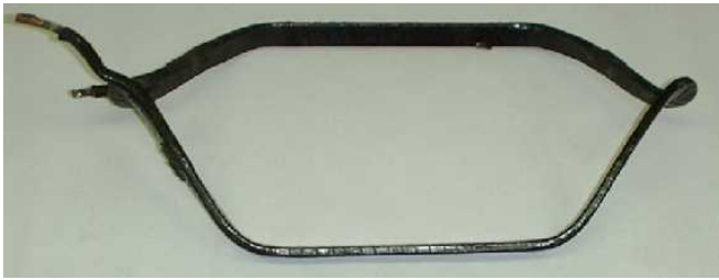
Figure 4. Shows one coil after being removed from the stator.
