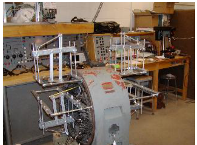
Figure 7. Test setup to measure inductance in slot sections.
