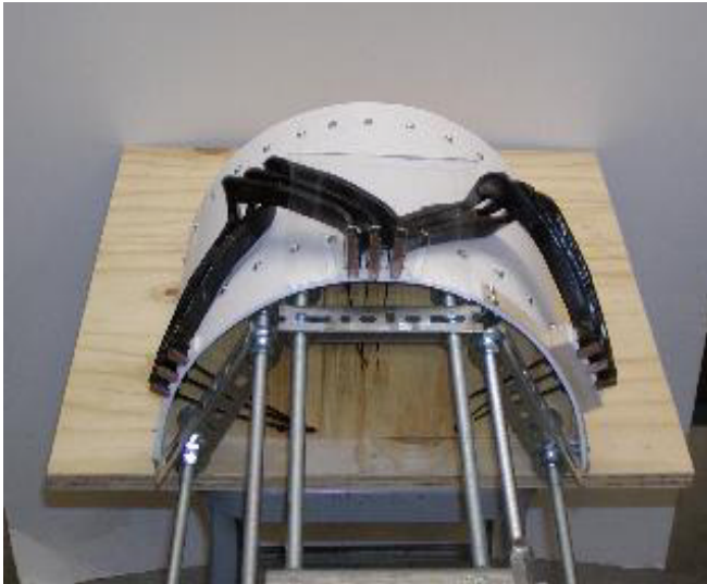
Figure 9. Form to hold overhang sections in proper alignment.
