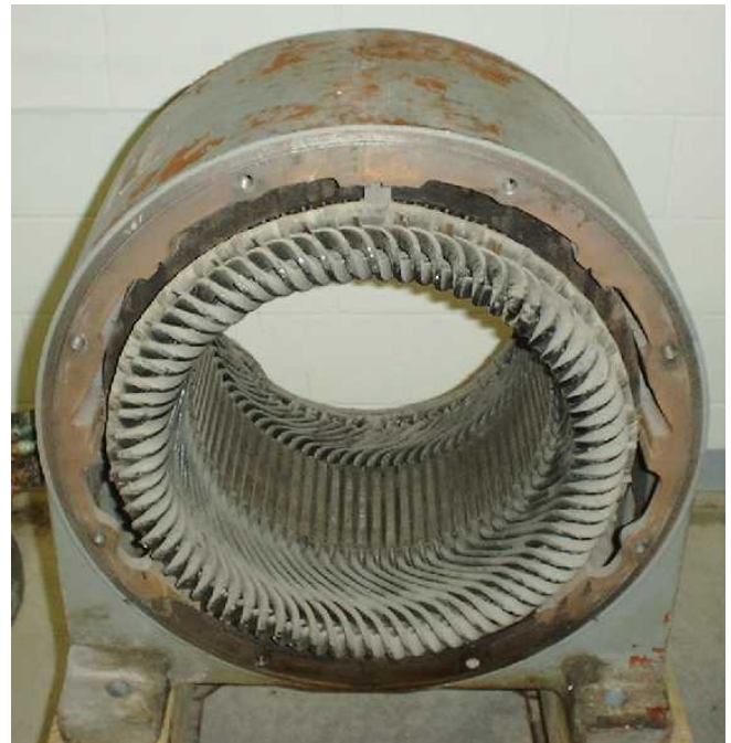
Figure 3. 150 HP, 3-phase, form wound induction motor used as test motor.
