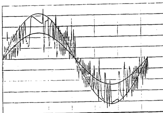
Figure 4. Delta current control with the motor as load A) experiment B) simulation.
