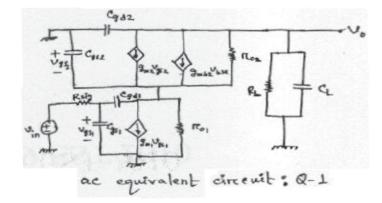
$V_{gs2} = V_g - V_{s2} = 0 - V_{s2}$  $V_{bs2} = V_b - V_{s2} = 0 - V_{s2}$
