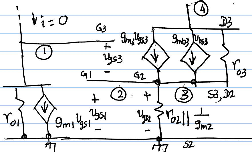
$$\text{From } g_m = \mu C_{ox} \frac{W}{L} (V_{GS} - V_{TH}) \\ = 100 \times 10^{-6} \times 10 \times 1 = 10^{-3} \text{ mho}$$
