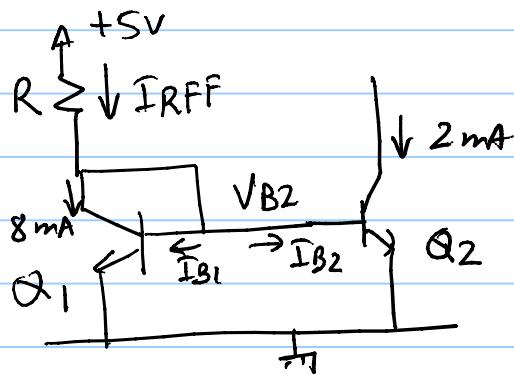
$$V_{BE2} = V_{B2} = V_T \ln\left(\frac{2 \text{ mA}}{0.25 \times 10^{-14} \text{ A}}\right) \\ = 0.025 \times 27.41 = 0.685 \text{ V}$$
