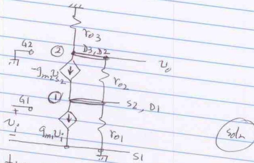
(b) This is a two node system with  $v_i$  as input node. Since  $v_i$  does not have any component attached, we will exclude it in formulating the nodal admittance matrix (NAM). By inspection (and letting  $g = \frac{1}{r}$ )
