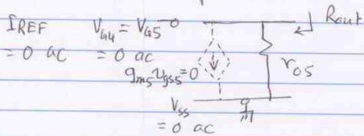
For (b), remembering  $I_{REF}$  is a DC value i.e. zero 'ac' the ac equivalent circuit will be:
