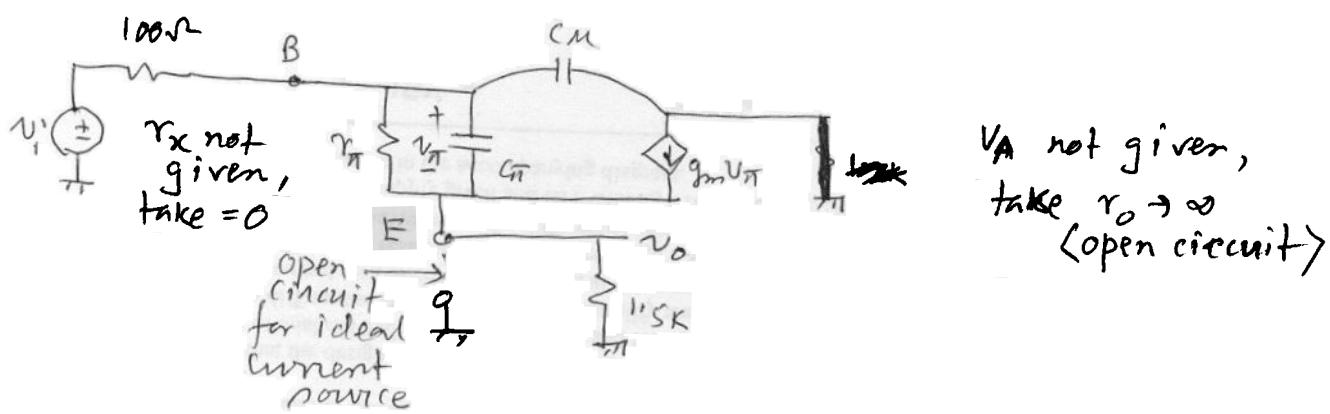
$V_i$  in series with  $100\Omega$  can be transformed to
