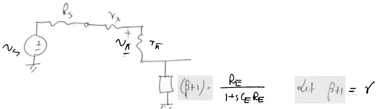
$$\begin{aligned} \text{Then } V_\pi &= \frac{r_\pi}{R_s + r_x + r_\pi + r} V_s \\ &= V_s \frac{r_\pi (1 + sC_E R_E)}{(1 + sC_E R_E)(R_s + r_x + r_\pi) + r R_E} \end{aligned}$$
