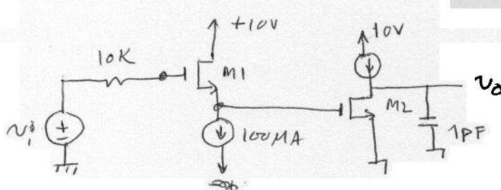
$$I_{DC} = 50 (V_{GS} - V_{TH})^2 \text{ mA} \\ = 100 \text{ mA for M1}$$
