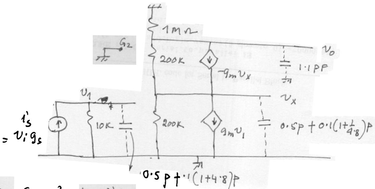
There are 3 possible O.C.T.C values at nodes  $v_1, v_x, v_o$  respectively
