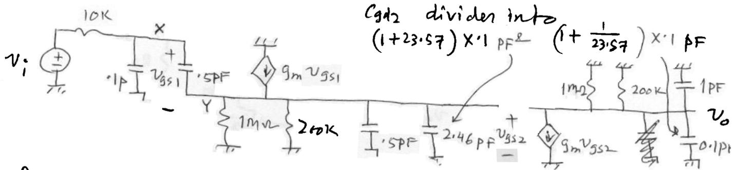
Between nodes X and Y, the CD amplifier has a voltage gain of  $\approx 1$ . We can apply Miller's Theorem to convert further
