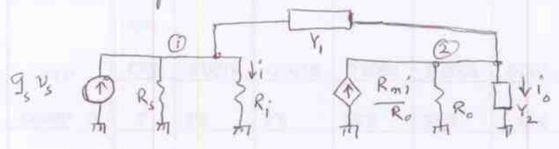
$$\begin{pmatrix} g_s + g_i + Y_1 & -Y_1 \\ -Y_1 & Y_1 + g_o + Y_2 \end{pmatrix} \begin{pmatrix} v_{\text{①}} \\ v_{\text{②}} \end{pmatrix} = \begin{pmatrix} g_s v_s \\ \frac{R_m}{R_o} i \end{pmatrix}$$
