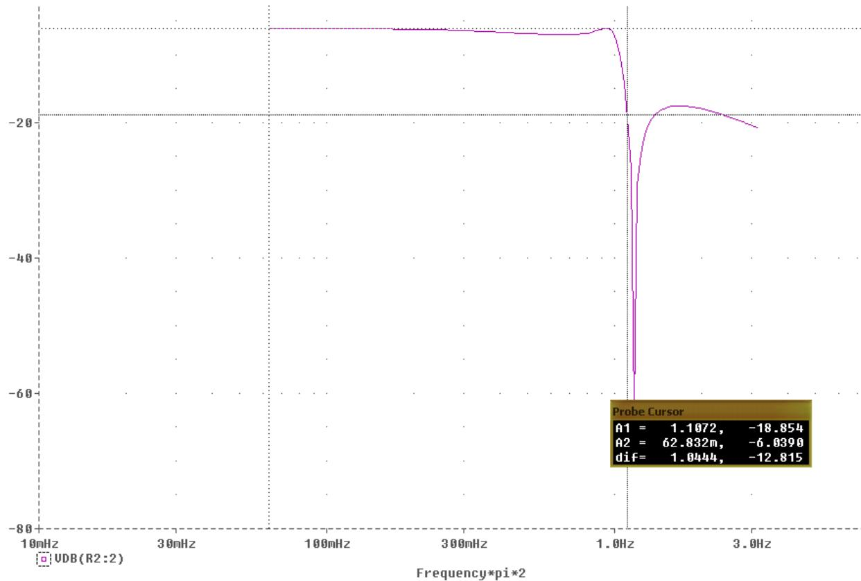
OTA-C based realization of the Elliptic LPF (text book Ch.7, p.243-245). The OTAs are simulated by ideal VCCS elements (SPICE symbol G). So each OTA input is shunted by  $10^{12} \Omega$  to avoid problems of 'open circuit' error messages.
