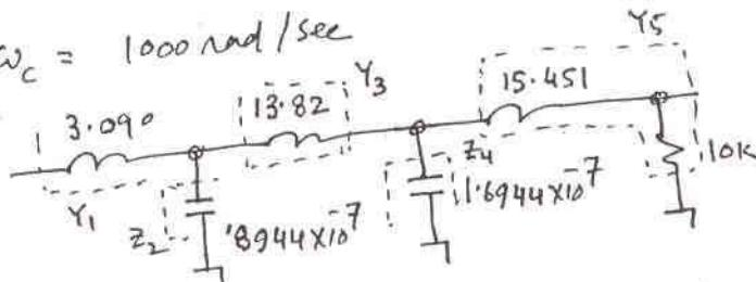
The branch gain functions are, successively, (See Fig. 14, eqn set 8(a))
