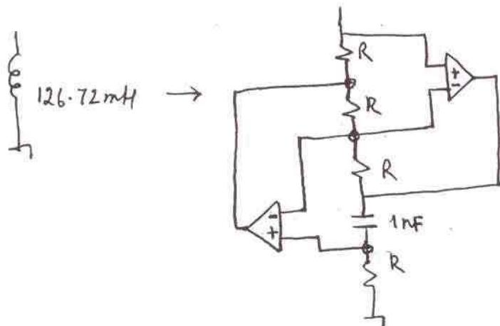
$$\begin{aligned} Z_{in} &= \frac{Z_1 Z_3 Z_5}{Z_2 Z_4} \\ &= SCR^2 \quad \text{if } Z_1 = Z_3 = Z_2 = Z_5 = R \\ Z_4 &= 1/SC \end{aligned}$$
