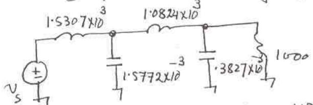
For a 3dB freq. of 500Hz,  $\omega_c = 2\pi \times 500$ . The LP  $\leftrightarrow$  HP transformation will give the HPF.
