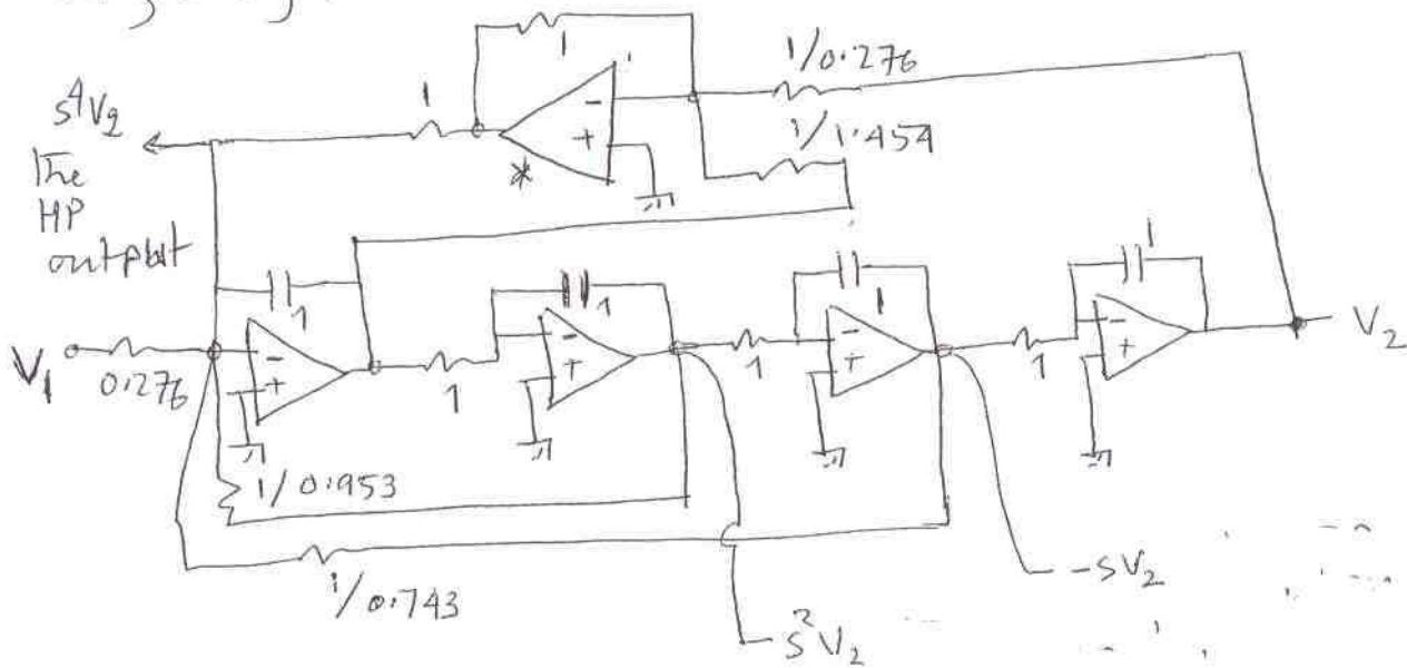
The HP output is obtained at the output of the inverting summer marked with an  $\ast$ .
