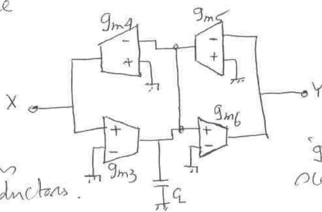
The floating inductor  $L_{xy}$  between XY is generated by  $C_L$  where  $Q = g^2 C_L$ . 'g' is a convenient scaling transconductance.
