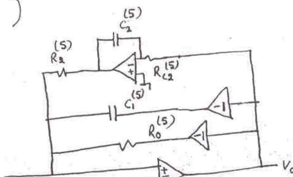
$$R_0^{(5)} = \frac{R_a R_p}{R_5}$$
