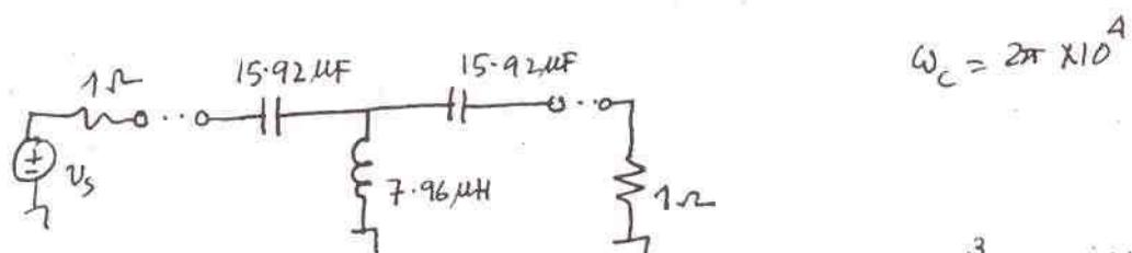
If all caps  $\rightarrow 1\text{nF}$ , divide  $15.92\text{μF}$  by  $15.92 \times 10^3$ , multiply  $7.96\text{μH}$  by  $15.92 \times 10^3$ , multiply  $R_s, R_L$  by  $15.92 \times 10^3$ .
