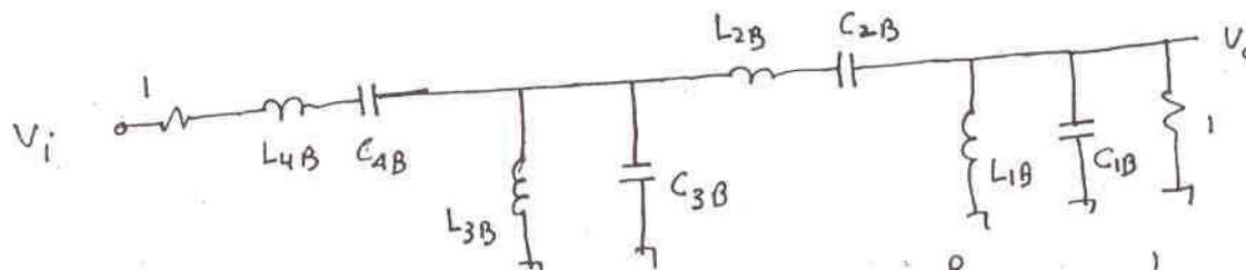
$$\left. \begin{aligned}L_{4B} &= \frac{L_4}{B} = L_4 \\C_{4B} &= \frac{B}{L_4 \omega_0^2} = \frac{1}{L_4}\end{aligned} \right\} \quad \left. \begin{aligned}L_{3B} &= \frac{B}{\sqrt{\omega_0^2 C_3}} = \frac{1}{C_3} \\C_{3B} &= C_3\end{aligned} \right\}$$
