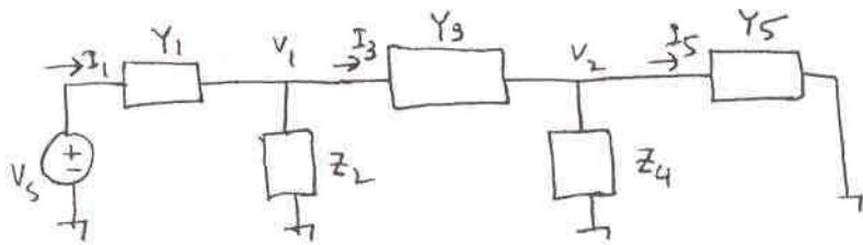
$$I_1 = (V_s - V_1) Y_1 ; \quad V_1 = (I_1 - I_3) Z_2$$
