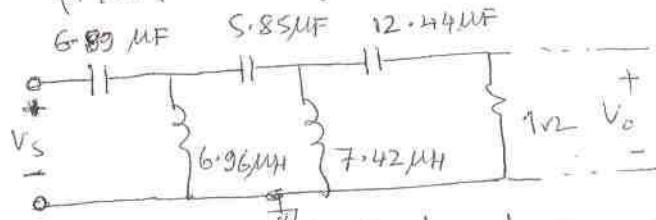
Because of grounded inductors, GIC-s with only one capacitor can be used to replace the inductors.
