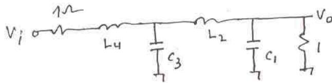
$$\begin{aligned}L_4 &= 0.7654 \\C_3 &= 1.8478 \\L_2 &= 1.8478 \\C_1 &= .7654\end{aligned}$$
