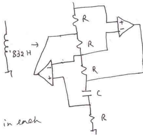
$$\therefore Z_{in} = S^2 R^2 \text{ with } R = 10\text{ k}\Omega \text{ in each case}$$
