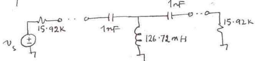
One needs to realize the  $126.72\text{mH}$  inductance by GIC. The capacitors in GIC have to be  $1\text{nF}$ .
