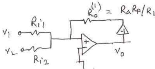
For  $t_{y3}$ ,  $R_a Y_1 T_1 \rightarrow sL_3 / R_p$ . Let  $Y_1 = SC_1$ ,  $-T_1 = -1$ , then  $R_a S C_1 = \frac{sL_3}{R_p}$
