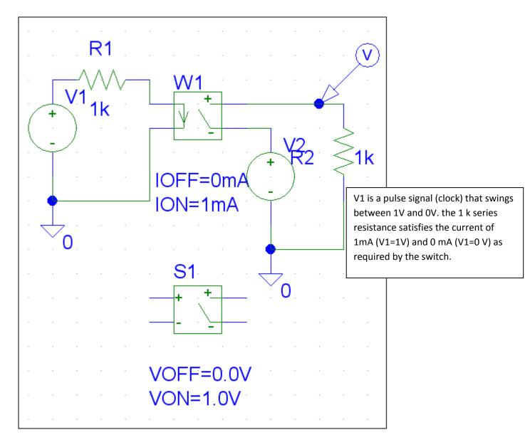
In PSpice, you may use a current controlled switch, such as 'W' device, or a voltage controlled switch, such as 'S' device above. Again try to satisfy the ON,OFF criteria of the switch as indicated with the switch schematic.
