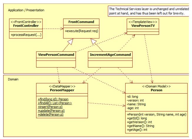
Figure 3-14 Using a FRONT CONTROLLER and COMMANDS to replace PAGE CONTROLLERS
