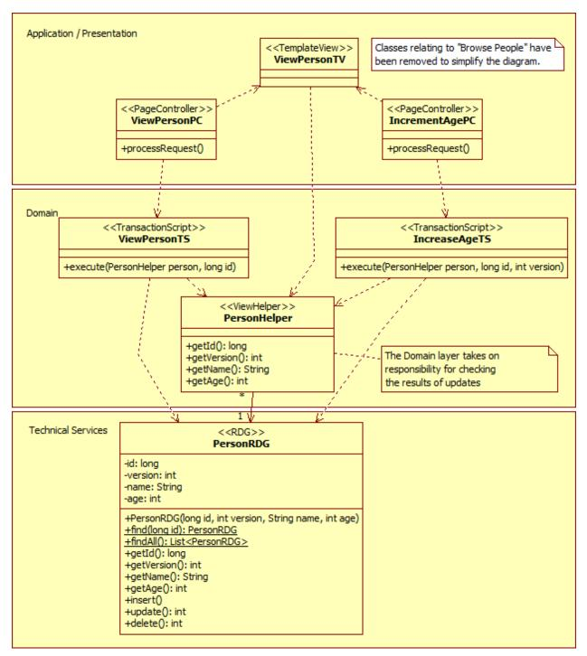
Figure 3-8 A class diagram showing PAGE CONTROLLERS, IDENTITY FIELD and OPTIMISTIC OFFLINE LOCK
