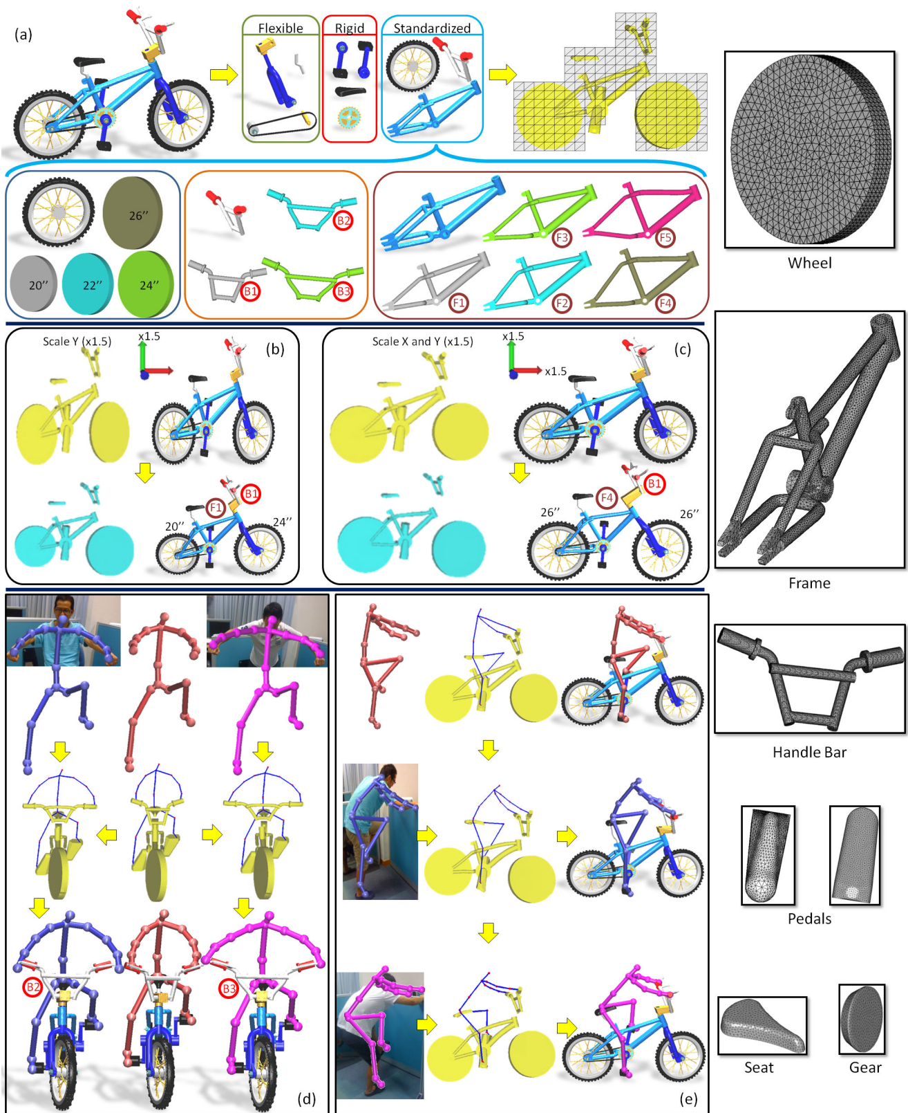
Figure 8: An illustration of using our MI-ARAP shape optimization framework for customizing bicycles: (a) A bicycle is constructed by flexible, rigid and standardized components and the volumetric meshes of different components are shown in the right, (b) a result of shape optimization for customization driven by simply scaling y-coordinates, (c) different result can be obtained by scaling both x- and y-coordinates, (d) results of customization driving by skeletons of users captured by Kinect sensors, and (e) another view for the results of skeleton-driven bicycle customization.
