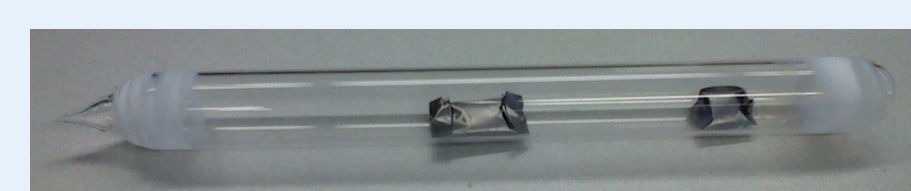
Figure 5: Samples inside a sealed quartz tube
