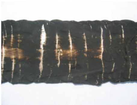
FIGURE 11: Black layer of coating on strip cast without protective atmosphere.
