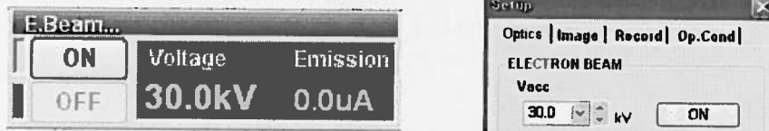
Fig. 3.3-2 Applying the Accelerating Voltage (a)
