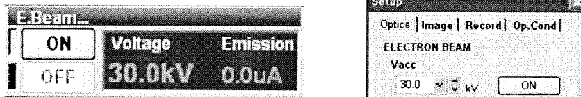
Fig. 3.3-2 Applying the Accelerating Voltage (a)
