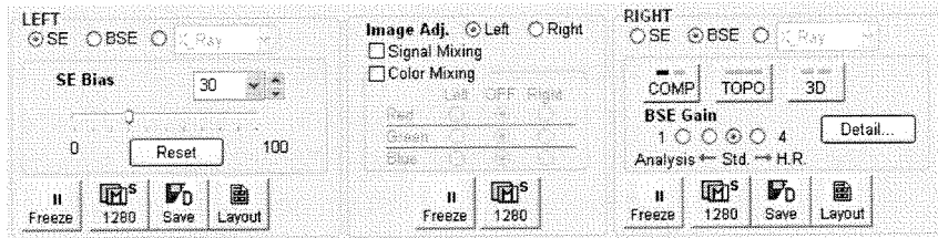
Fig. 3.9-10 Enhanced Control Panel for Dual Mode
