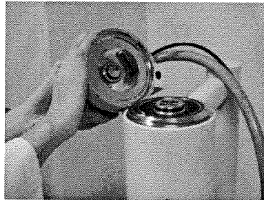
Fig. 4.1-35 Removing the Electron Gun Unit
