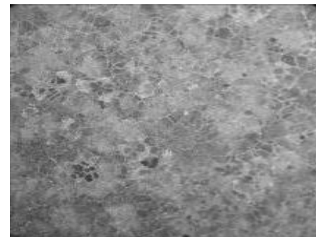
Figure 3: Photomicrograph of the general microstructure of ZA5+0.04%Hf, X200
