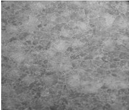
Figure 5: Photomicrograph of the general microstructure of ZA5+0.08%Hf, X200
