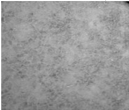
Figure 6: Photomicrograph of the general microstructure of ZA5+0.10%Hf, X200
