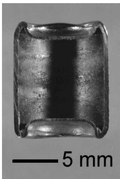
Fig. 1 Cross section of an empty Ta crucible demonstrates the smoothly welded bottom and lid. The DTA thermocouple tip will touch the concave bottom part which is only 0.25 mm thick
