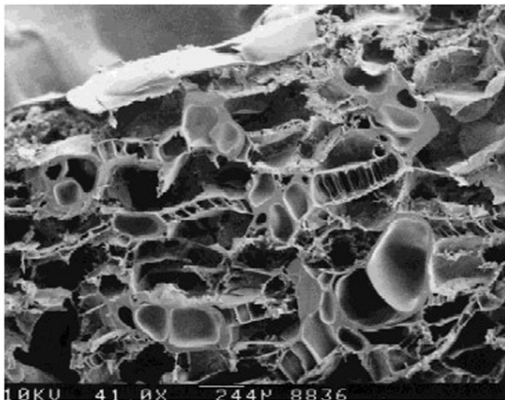
Figure 3.3 High magnification scanning electron photomicrograph of gas foaming and particulate leaching matrix demonstrating macropores, formed by leaching of NaCl particles, and smaller pores formed by the gas pores within the polymer particles.
