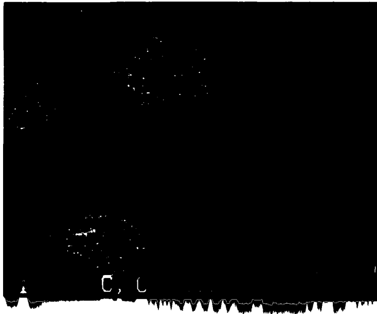
Fig. 3.22. Carbon compositional map for cross section of SiC/Vitreloy™ 1 composite. Image taken with SAM. Sample infiltrated for 0.5 h.
