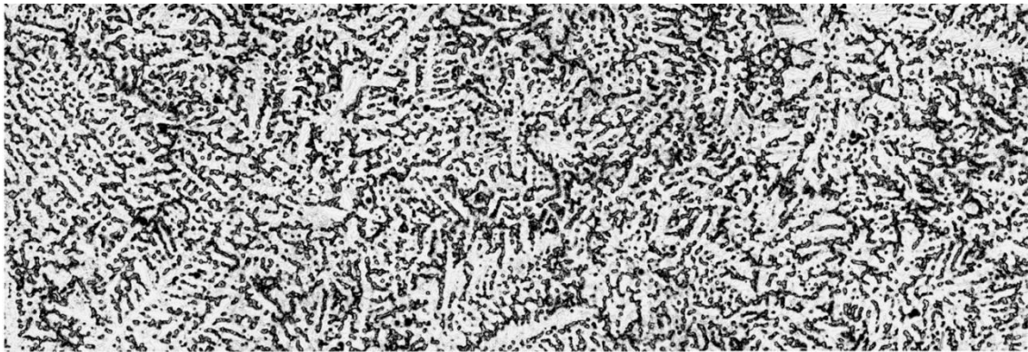
Figure 5-8: Columnar to equiaxed transition
