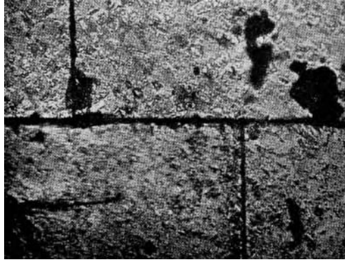
Figure 6.64 Grain boundary sliding on a bi-crystal tin (after Puttick and King, 1952; courtesy of Institute of Materials, Minerals and Mining).
