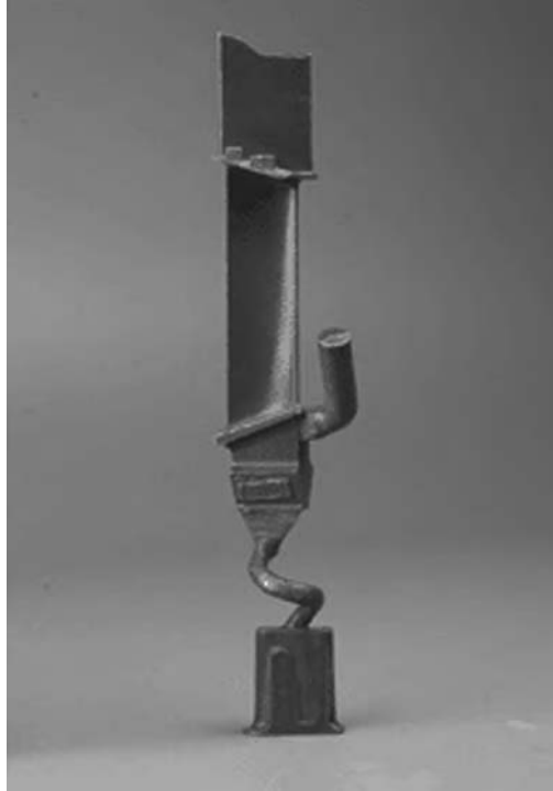
Figure 2.6 A single-crystal blade embodying a DS starter block and helical constriction, and a test plate facilitating orientation check by XRD (Courtesy of Prof. H. K. D. H. Bhadeshia).
