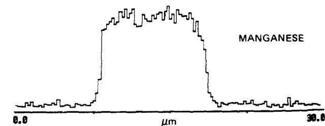
Fig. 7. (a) Electron micrograph and (b) composition profiles of a Pr-66.6at.%Mn alloy annealed at 700 °C for 150 h and at 600 °C for 700 h and finally quenched in water. The composition profiles were taken along the section of the specimen indicated in the electron micrograph by the white line. The praseodymium and manganese contents are given in arbitrary units. It should be noted that the two phases are almost coincident with the pure metals. (Magnification: (a) 1800 \times .)
