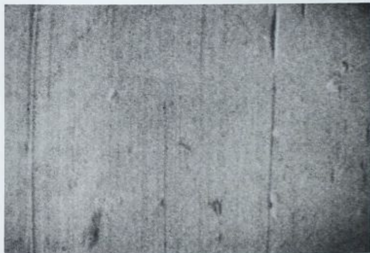
FIG. 16—Photomicrograph of 8-deg electroformed nickel dual-orifice nozzle—left side ( \times 675 ).
