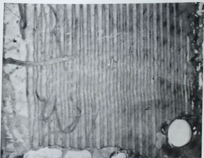
FIG. 5—Coated specimen cleaned and undamaged by waterjet.
