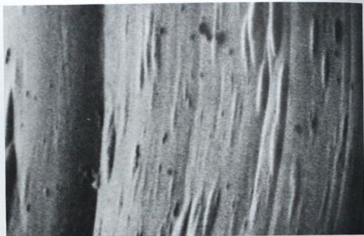
FIG. 10— Photomicrograph of the 2-deg dual-orifice nozzle—right nozzle ( \times 675 ).
