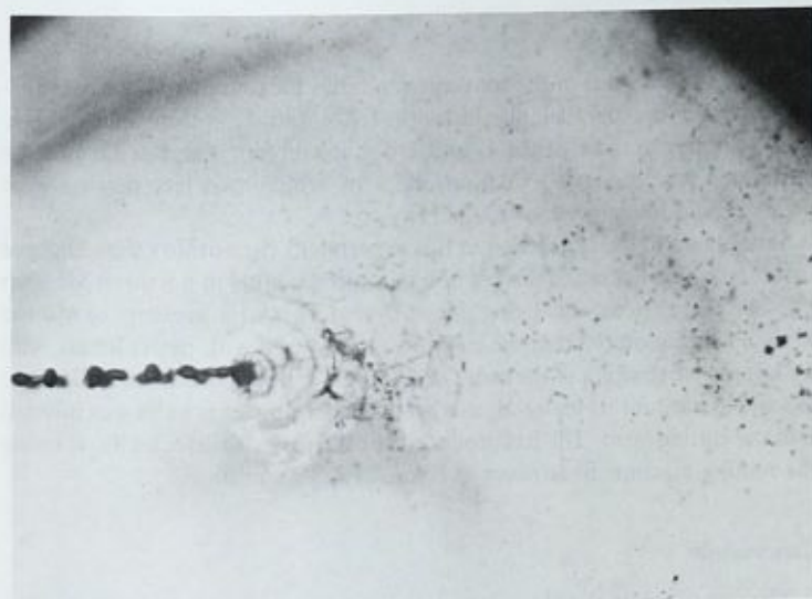
FIG. 12—Views of water jets at a pressure of 4 bar converging at an angle of 10 deg at the point where the jet turns into droplets: (a) top view showing the angle of impact, (b) side view showing shock waves generated by the small augmented jet velocity.
