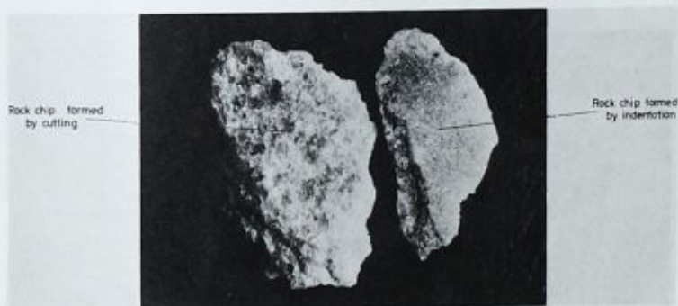
FIG. 4—Geometric similarity between rock chips formed during the cutting operation and those formed during indentation tests.
