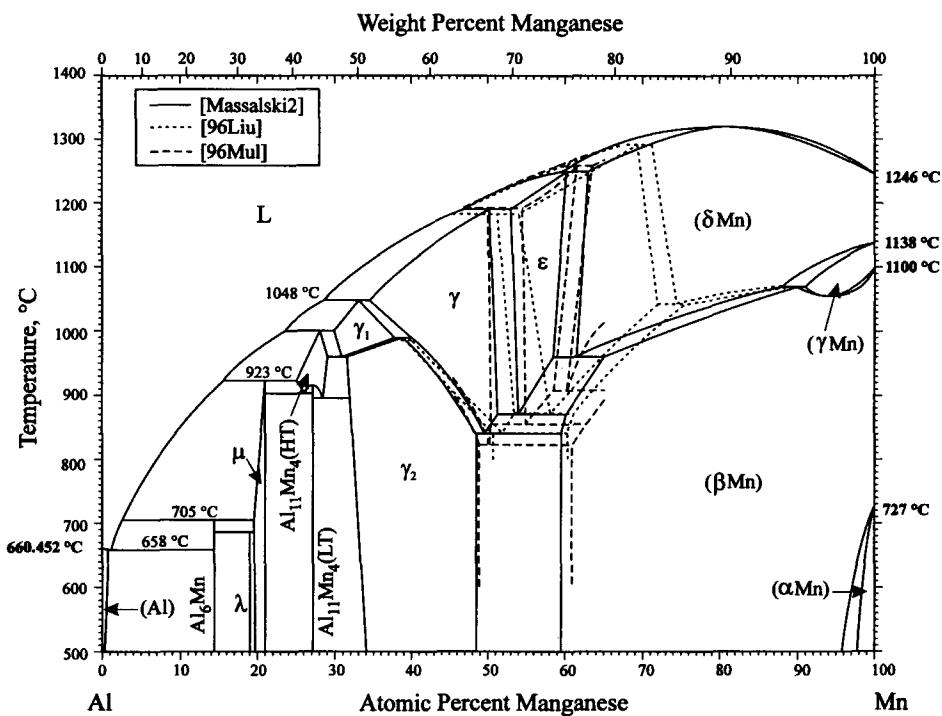
**Fig. 1** The Al-Mn phase diagram.
