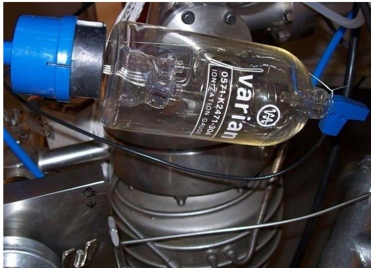
**Figure 19 X-ray enhanced hot cathode ionization gauge (Bayard-Alpert)**
