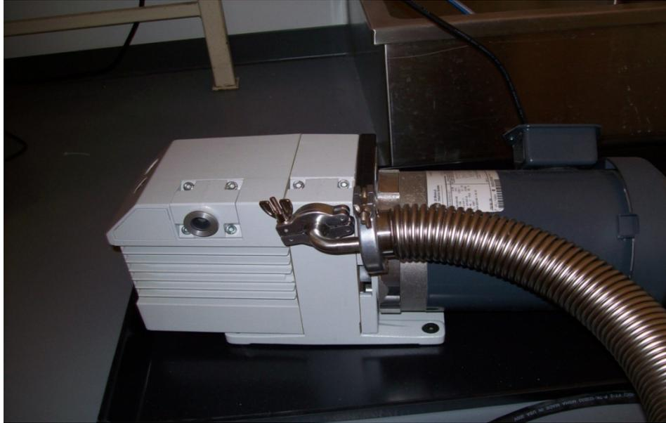
**Figure 13 Rotary vane type pump used for rough vacuum**
