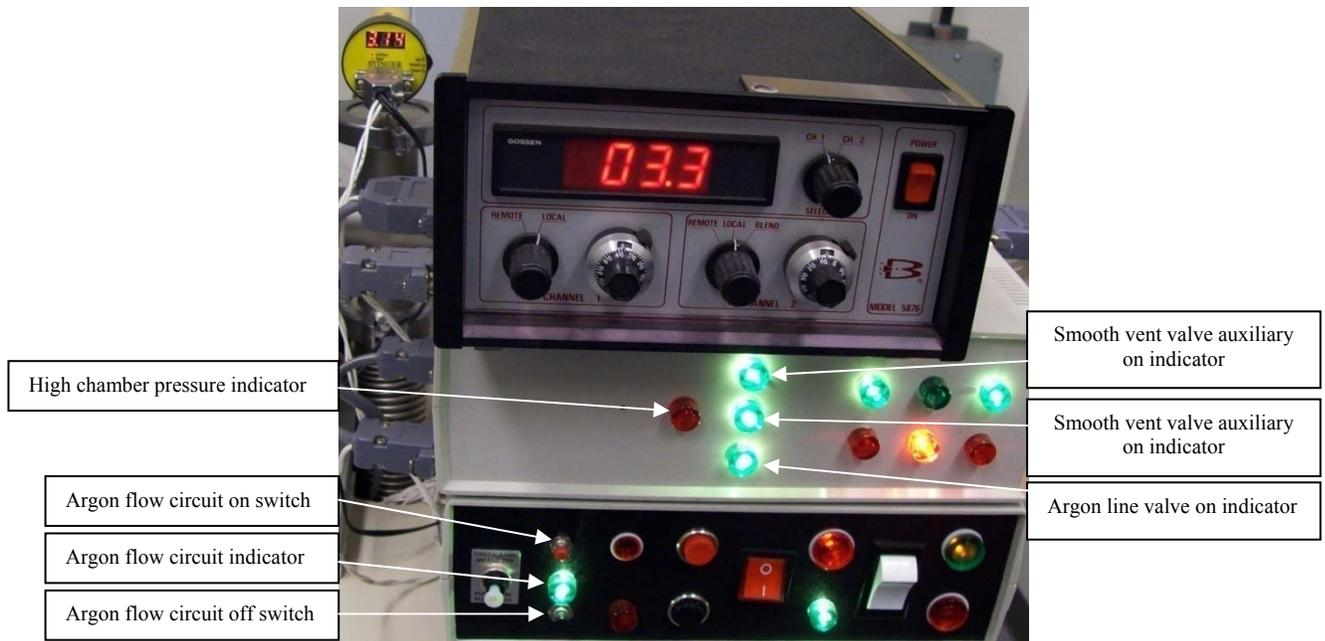
**Figure 48 View of the control panel during argon flow operation**
