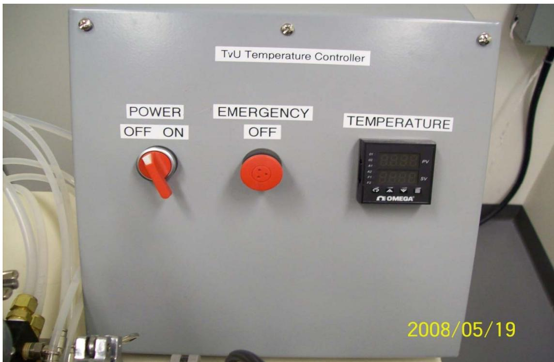
**Figure 11** External view of the furnace controller
