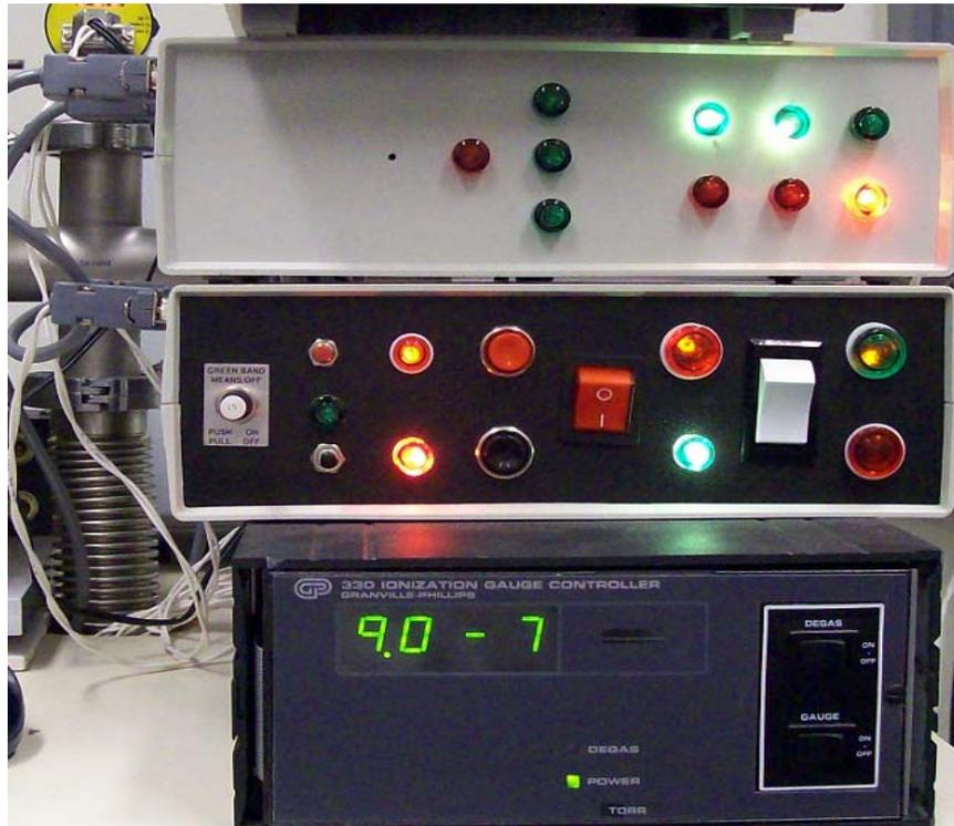
**Figure 29** View of the vacuum control panel during operation
