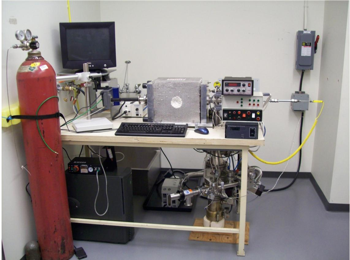
**Figure 27 View of the complete facility to monitor the spreading behaviour of the brazing filler metals at high temperature**
