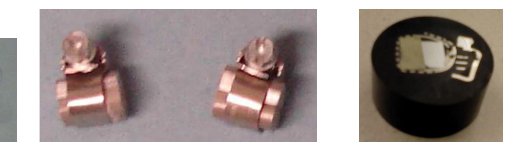
Figure 4: Clamped and Mounted diffusion couples
