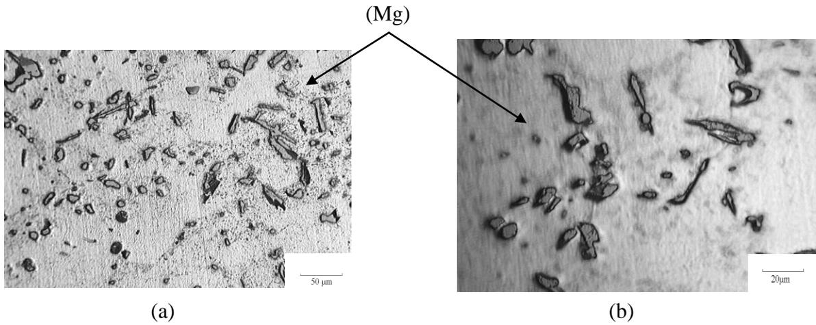
Figure 48: Post-DSC microstructure of AE44, DSC cooling rate 10°C/min, (a) 500X (b) 1000X
