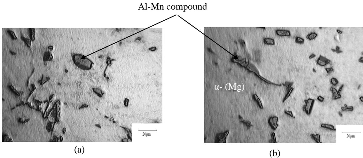
Figure 49: Post-DSC microstructure of AE44, DSC cooling rate 20°C/min, (a) 500X (b) 1000X
