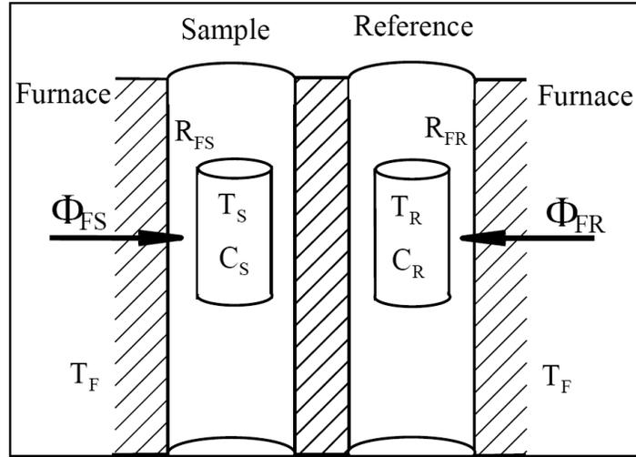
Figure 15: Schematic view of a heat flux DSC, with quantities used in the heat transfer model [53]
