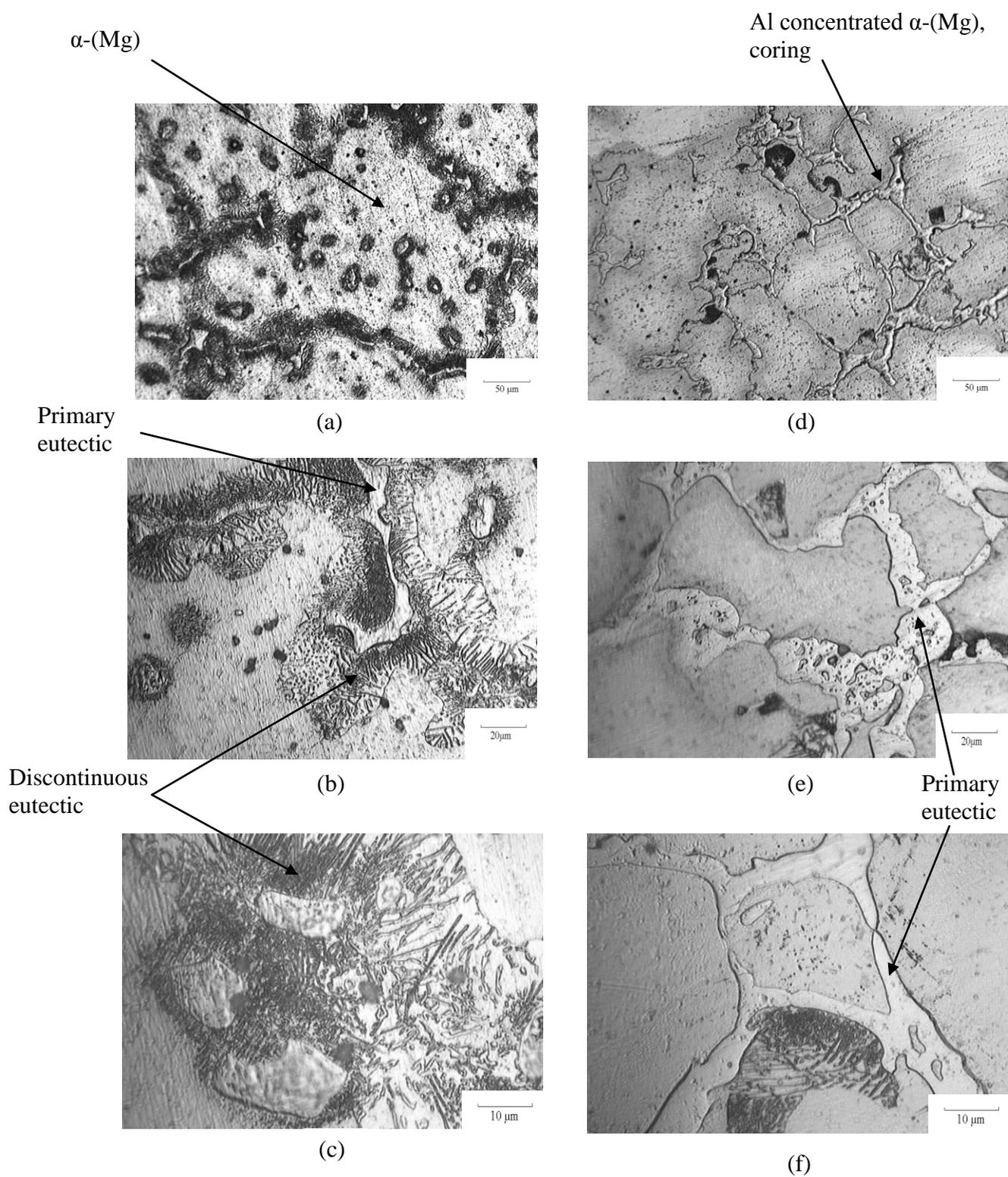
Figure 42: As-cast microstructure of AZ91D: (a)100X (b) 500X (c) 1000X; Post-DSC microstructure of AZ91D, DSC cooling rate 5°C/min: (d) 100X (e) 500X (f) 1000X.
