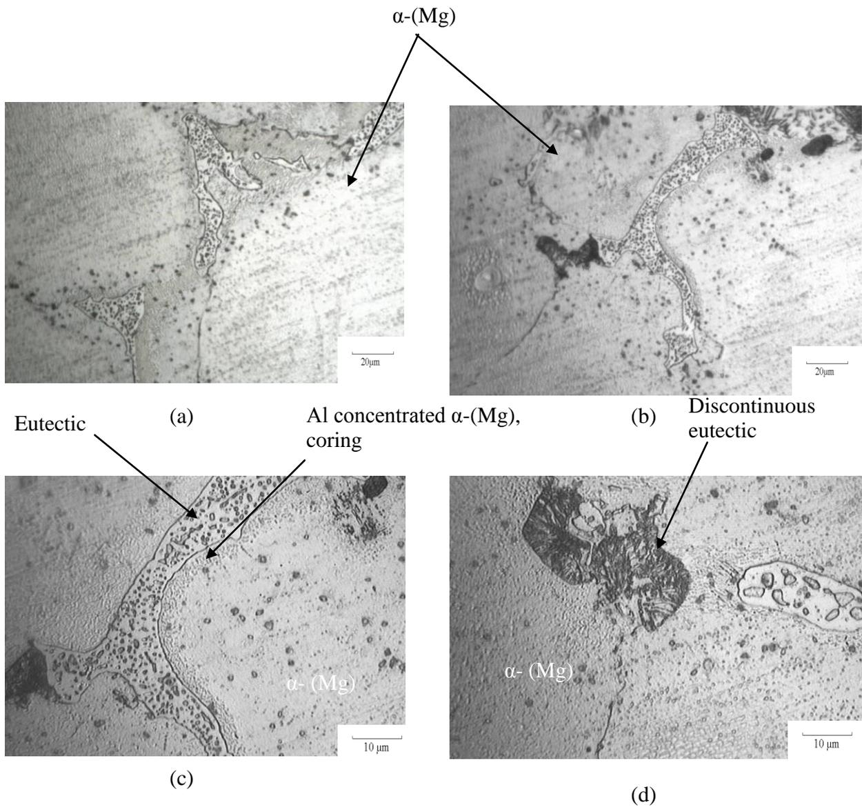
Figure 45: Post-DSC microstructure of AM60B, DSC cooling rate 5°C/min: (a) 500X (b) 500X (c) 1000X (d) 1000X
