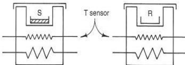
Figure 12: The principle of power compensated Differential Scanning Calorimeter Analysis [48]
