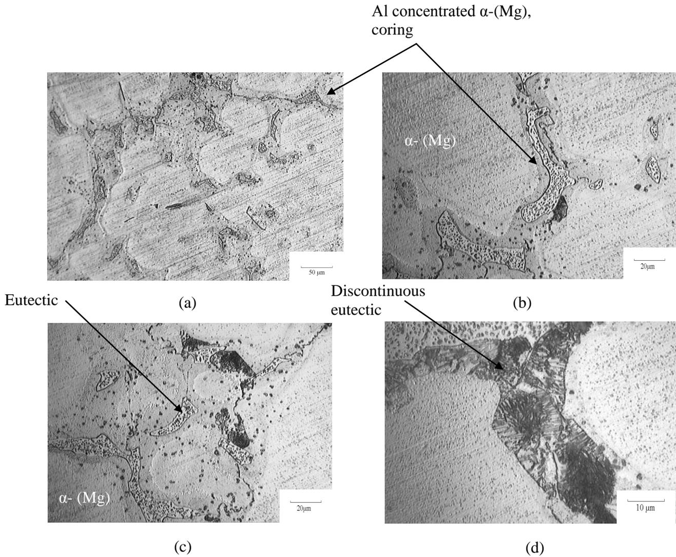
Figure 46: Post-DSC microstructure of AM60B, DSC cooling rate 45°C/min: (a) 100X (b) 500X (c) 500X (d) 1000X
