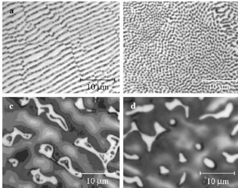
Figure 10: (a) Lamellar, (b) fibrous, (c) partially divorced and (d) fully divorced morphologies in Mg-Al alloys of various compositions [29]
