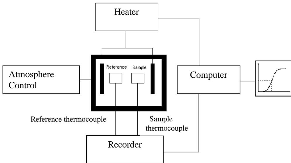
Figure 13: The principle of heat flux Differential Scanning Calorimeter Analysis [49]
