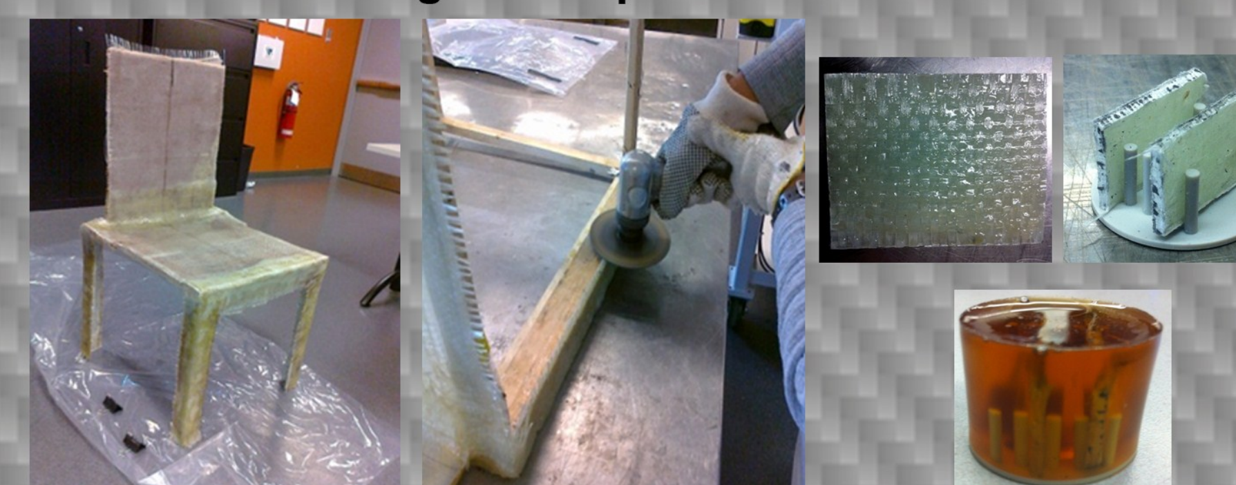
Figures 14-18: Applying all the composites laminates, trimming the excess edges and microscopic inspection
