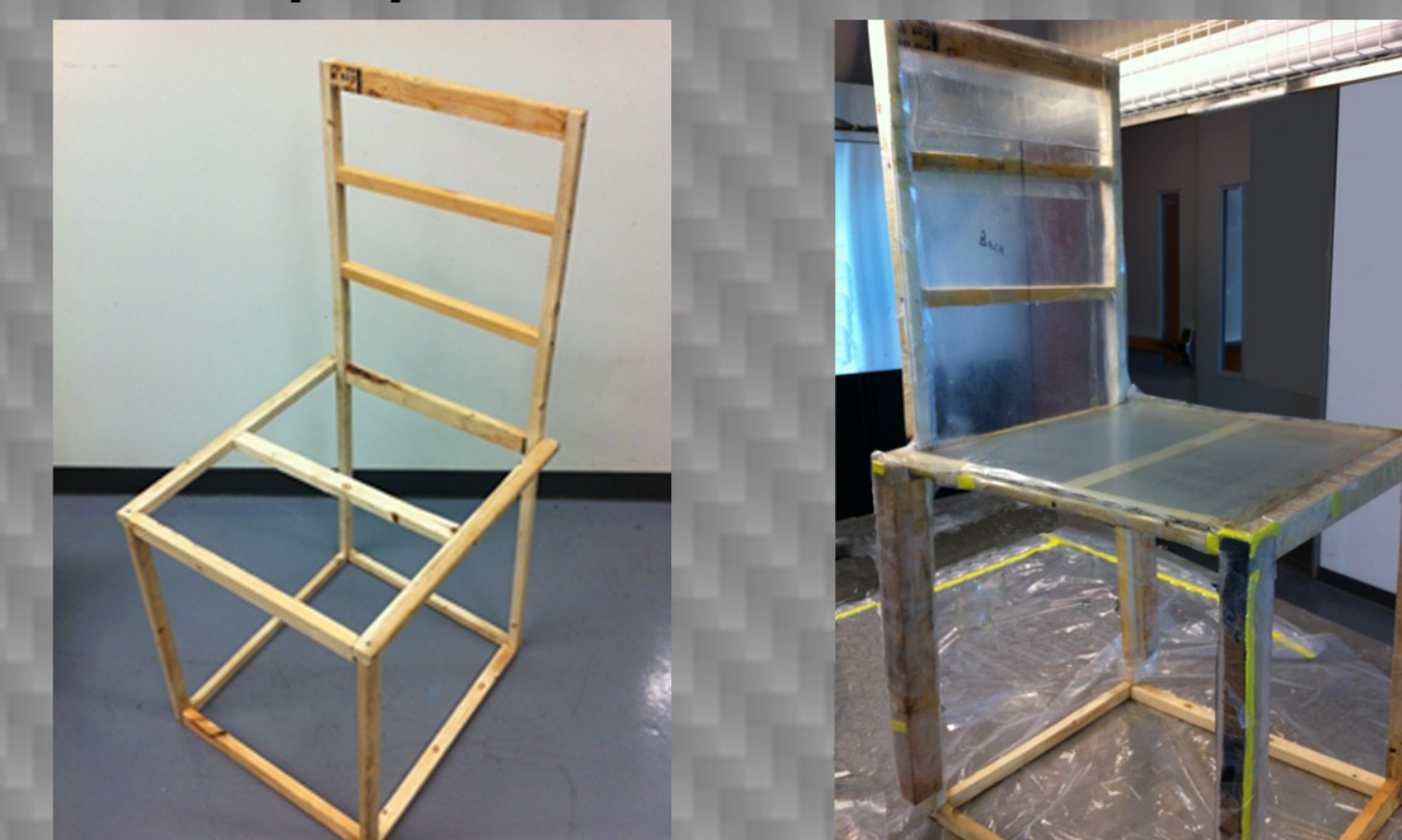
Figures 7, 8: Wooden mold preparation and plastic sheet covering
