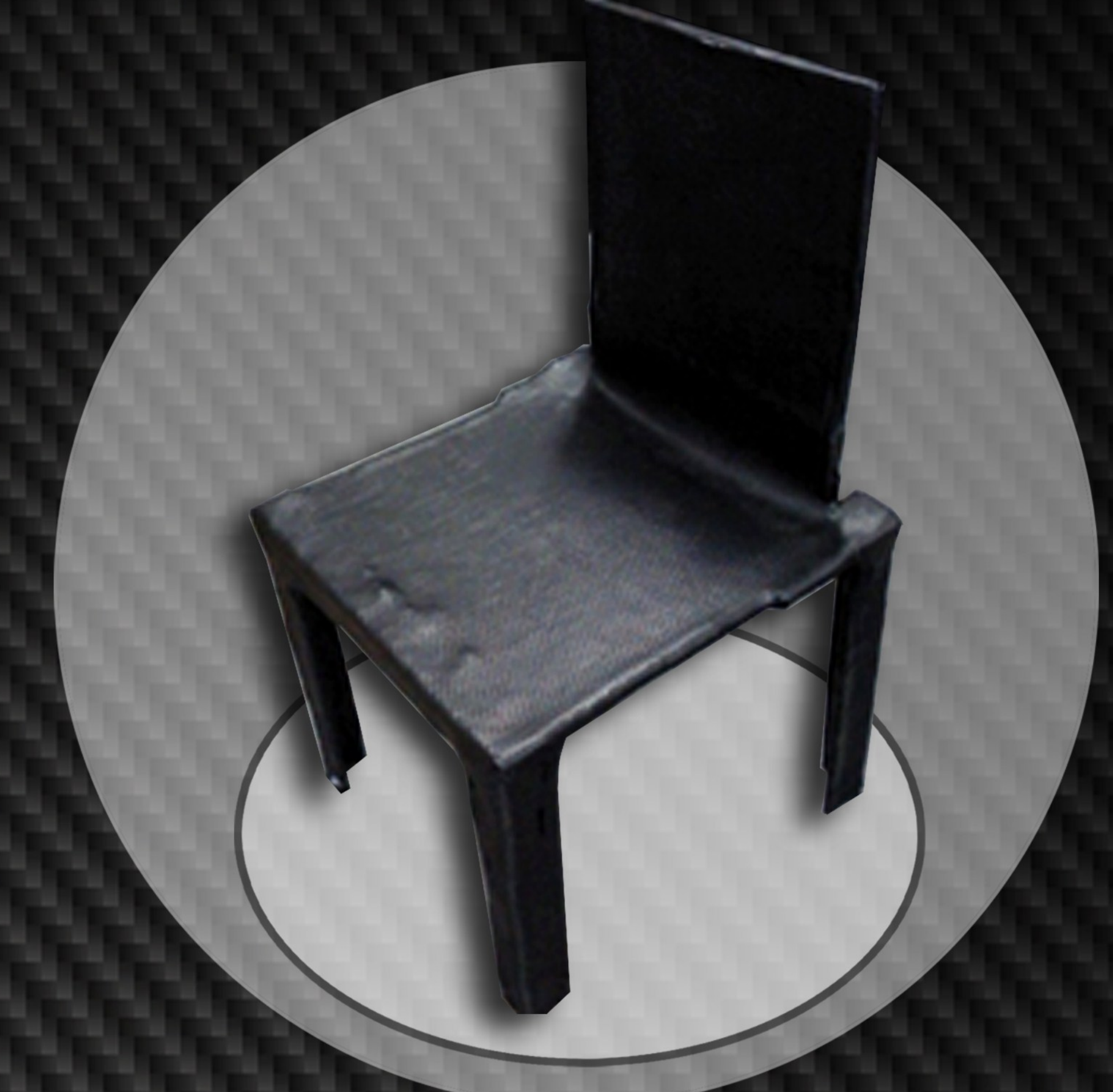
Figure 19: The final seat made of polyester resin/fiberglass composites
