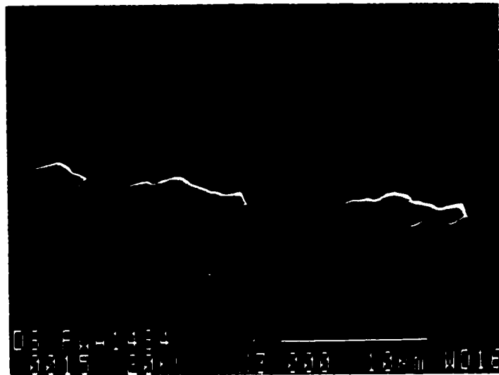
Figure 5-24 Small carbide chain along grain boundary observed in a sample grown at V=0.00005\text{cm/s}
