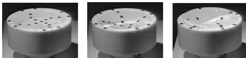
Figure 6.5: Side view of open cup experiment showing the three-dimensional deformation field present. Time history from left to right.
