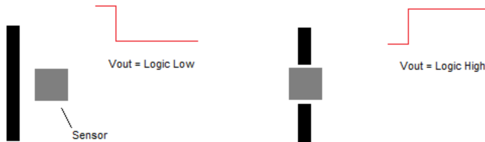
Figure 6.13: (left) Output voltage when away from black tape line, (right) Output voltage when over black tape line.
