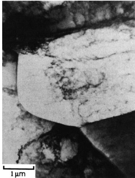
Fig. 7.28. TEM micrograph of SIBM in copper deformed 14% in tension and annealed 5 min at 234°C, (Bailey and Hirsch 1962).
