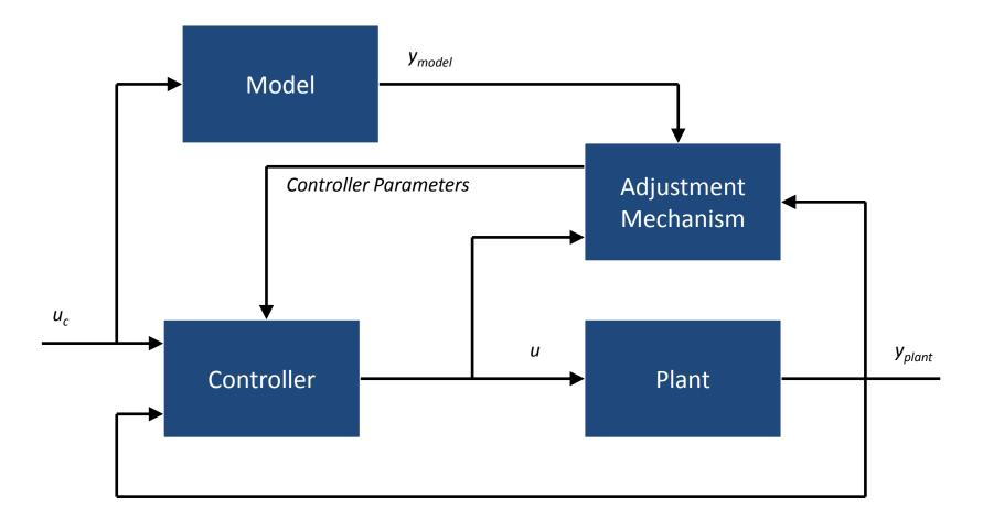
Design controller to drive plant response to mimic ideal response (error =  $y_{plant}$ - $y_{model} => 0$ ) Designer chooses: reference model, controller structure, and tuning gains for adjustment mechanism
