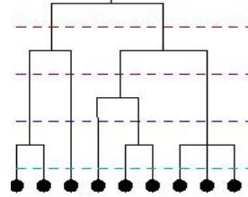
**Figure 2. A dendrogram with various cut points represented as dashed lines**
