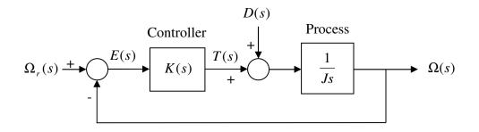
In the diagram,  $\Omega_r(s)$ ,  $\Omega(s)$ , T(s), and D(s) are the Laplace transforms of the reference speed, output speed, driving torque, and disturbance torque, respectively. *J* Problem Set Prepared by Amir G. Aghdam
