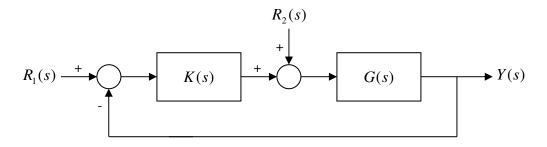
• Find the output of the system to the input  $r_1(t)$  when  $r_2(t) = 0$ . This output is denoted by  $Y_1(s)$  in the *s*-domain.
