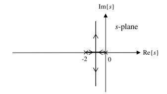
It can be easily seen that using a constant controller the desired specifications cannot be met (no complex poles on the trajectory will be inside the desired region).
