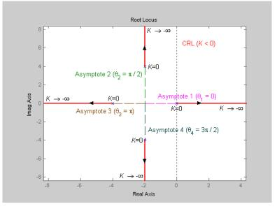
Note that the root loci are symmetrical w.r.t. the line  $\text{Re}\{s\} = -2$  (and the real axis) as this line is the axis of symmetry for the open loop poles.
