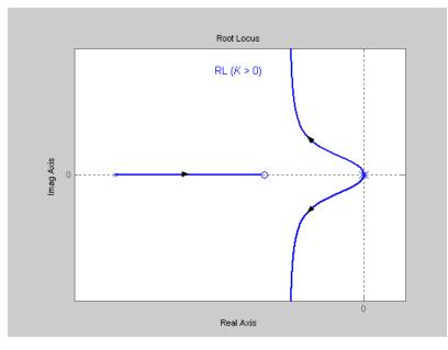
It is desired to find K, z and p, so that  $s_1, s_2 = -2 \pm j2$  be the dominant poles of the closed loop system.
