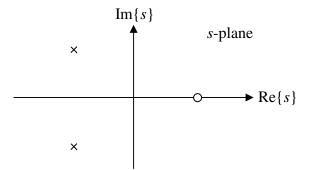
Assume that the zero of the loop transfer function is located at s = 1 and the poles are located at  $s_1$ ,  $s_2 = -1 \pm j$ . The RL for this example is given below.
