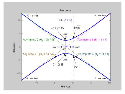
To find the point at which the trajectory crosses the imaginary axis, we can use the RH method as follows:
