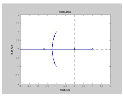
It is desired to find the angle of locus departure from the pole  $s_1 = -1 + j$ . Consider a point  $s_0$  on the RL, very close to  $s_1$  as shown below.
