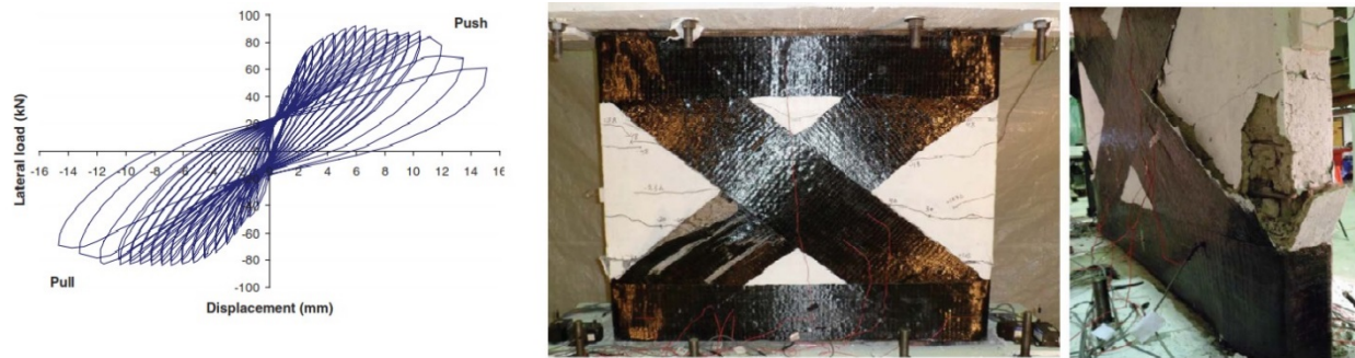
Figure 32: Lateral Load-top Displacement, Rupture of Diagonal FRP and Concrete Crushing and Buckling of Flexure Reinforcement of RW2 (El-Sokkary and Galal, 2013)
