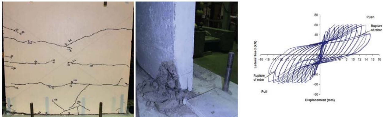
Figure 30: Crack Pattern at Failure, Concrete Toe Crushing and Lateral load-top Displacement of CW (El-Sokkary and Galal, 2013)
