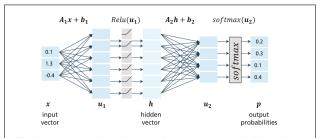
Fig. 1.1 A neural network for classification transforms the input by layers with affine transformations and nonlinear activation functions, e.g. ReLU. The final layer usually is a logistic classifier
