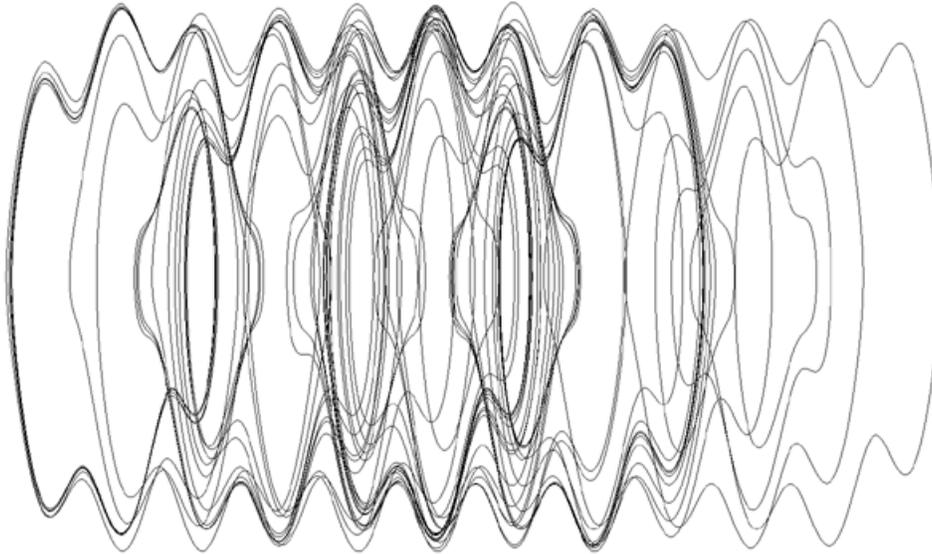
Figure 5: A single trajectory in the state space of a damped simple pendulum driven by a sinusoidal force.
