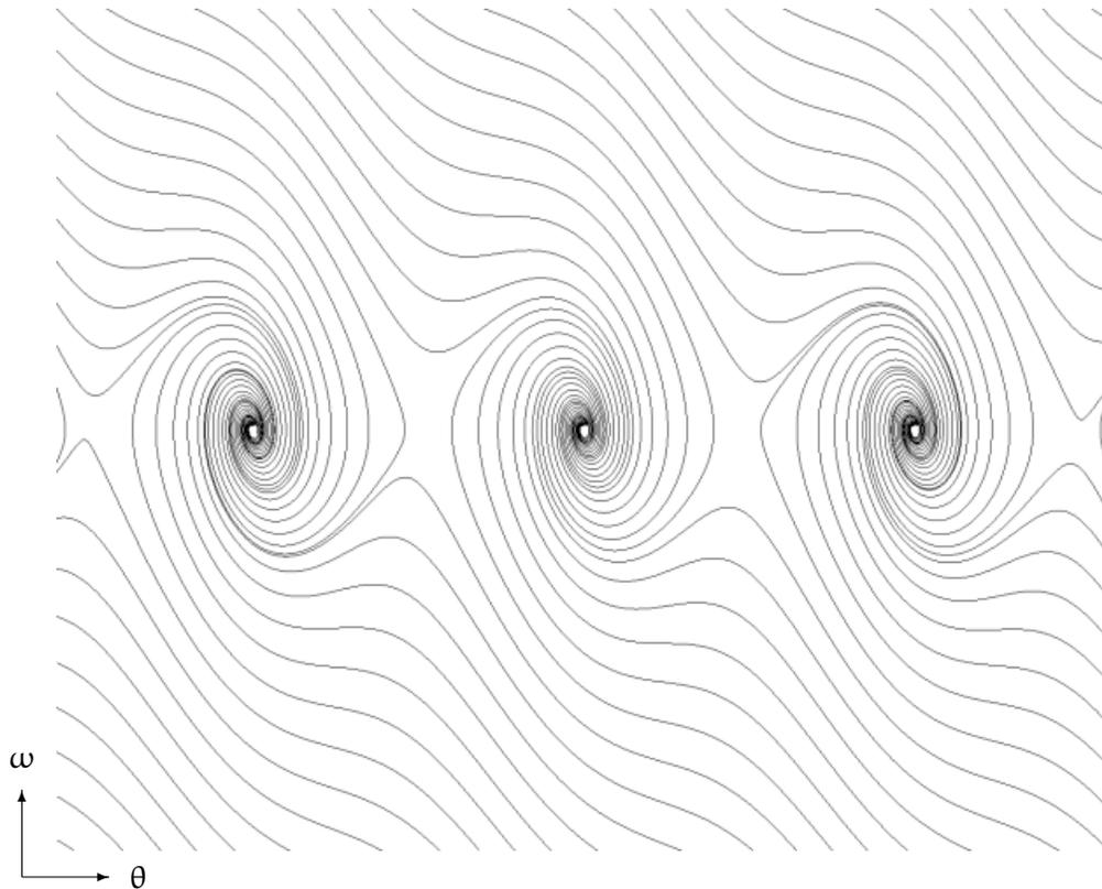
Figure 2: State space of the damped simple pendulum. The equation of motion is  $\ddot{\theta} + \dot{\theta} + 5 \sin \theta = 0$ .
