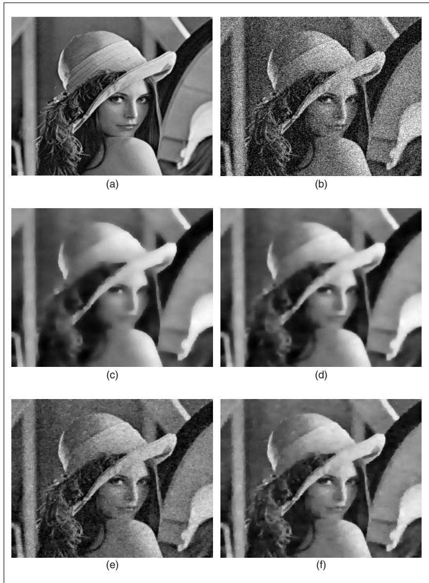
▲ 11. Filtering results for Gaussian noise: (a) original image, (b) noisy image, (c) Huber, (d) entropic, (e) total variation, and (f) improved entropic.
