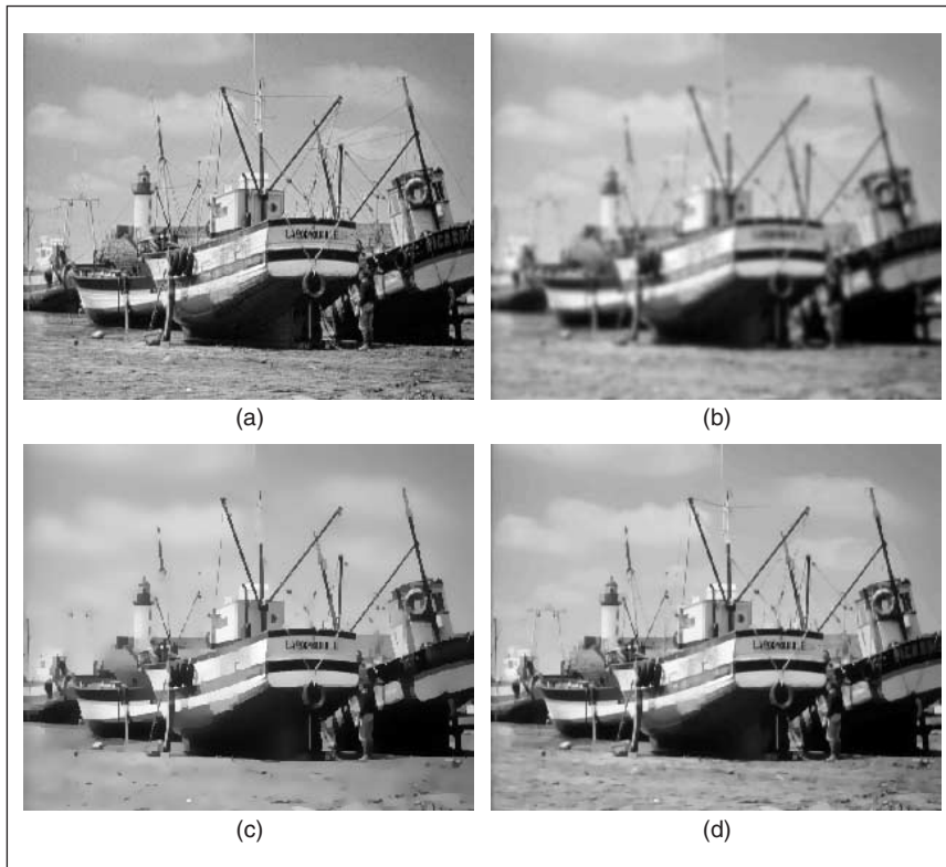
▲ 4. Filtering results: (a) original image, (b) heat flow, (c) Perona-Malik flow, and (d) TV flow.
